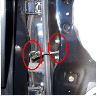
4) You will need to remove the door panel: Remove all the covers and screws, you will find (2) on the bottom side of the arm rest and (2) under the cover of the door handle.
