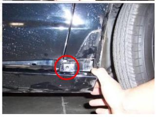
Open the door and remove (1) 10mm bolt located at the point where the windshield pillar meets the fender.
