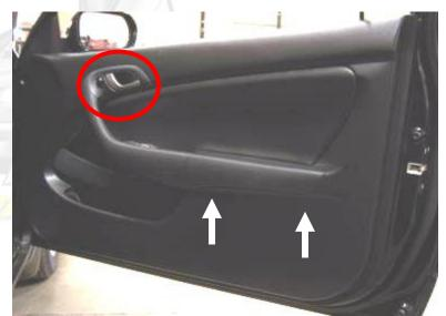
After removing the two screws under the door handle cover you will be able to pull the assembly out and disconnect the cable that opens the door and the wire harness that control the lock.
