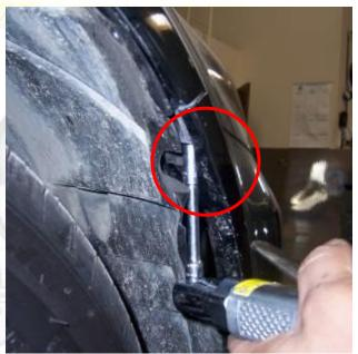
After removing the 10mm bolt, pull back on the bumper to gain access to (2) 10mm bolts securing a plastic bracket. After removing the top bracket remove the other (2) bolts securing the fender to the body.
